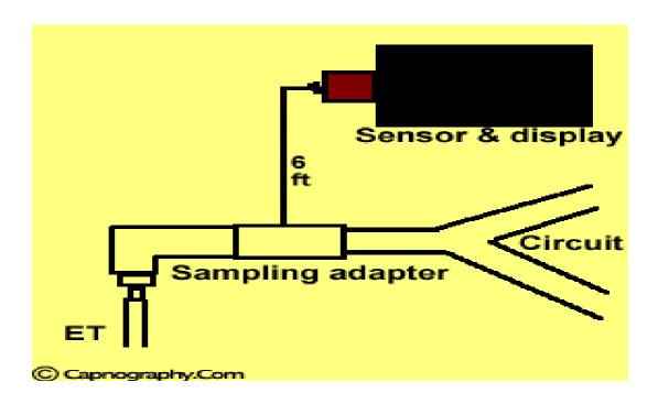
In this type, the CO 2 sensor is located in the Mainstream itself and a tiny pump aspirates samples from the patient's airway through a 6 feet long capillary tube into the main unit.
