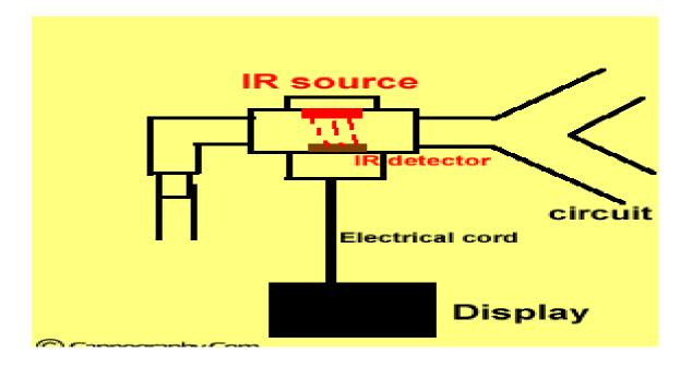
In the main stream capnograph , a cuvette containing the CO2 sensor is inserted between the breathing circuit and the endotracheal tube .
