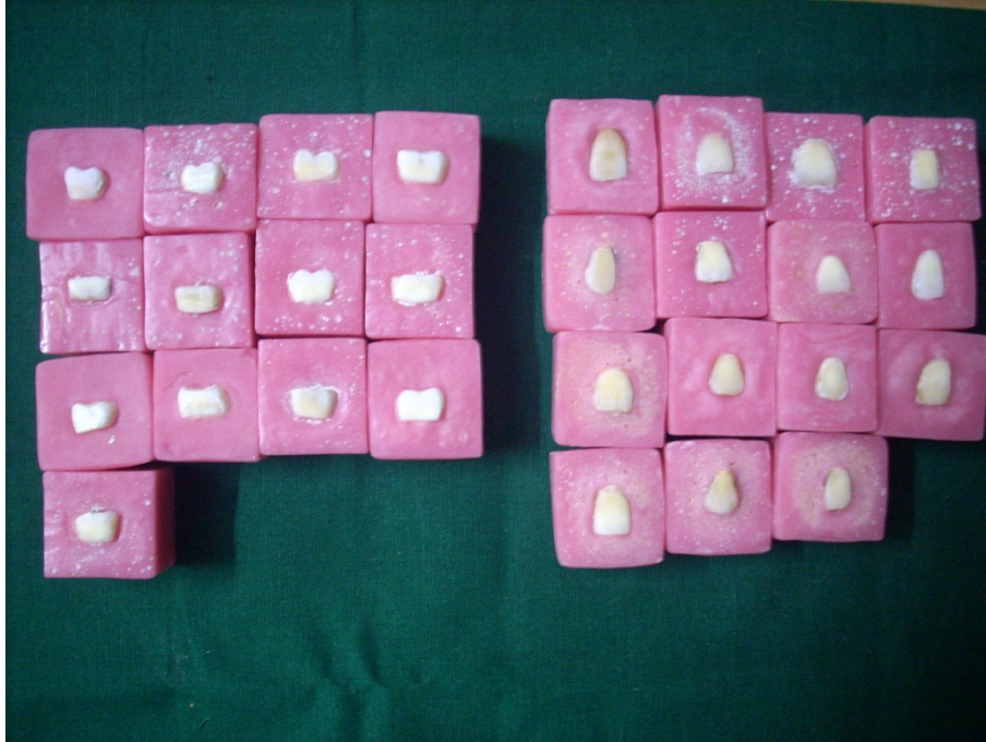
FIG. 5 TEETH SAMPLES EMBEDDED IN ACRYLIC BLOCKS
