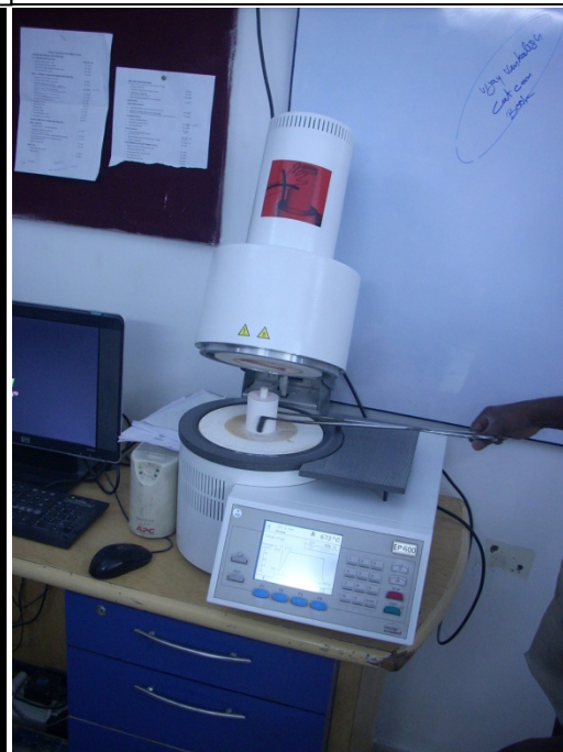
FIG. 17 PLACING RING WITH PLUNGER AND BUTTON INTO PRESSING MACHINE
