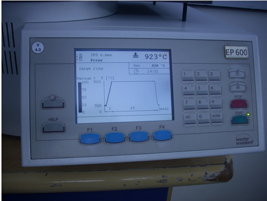
FIG. 18 PRESSING TEMPERATURE REACHED
