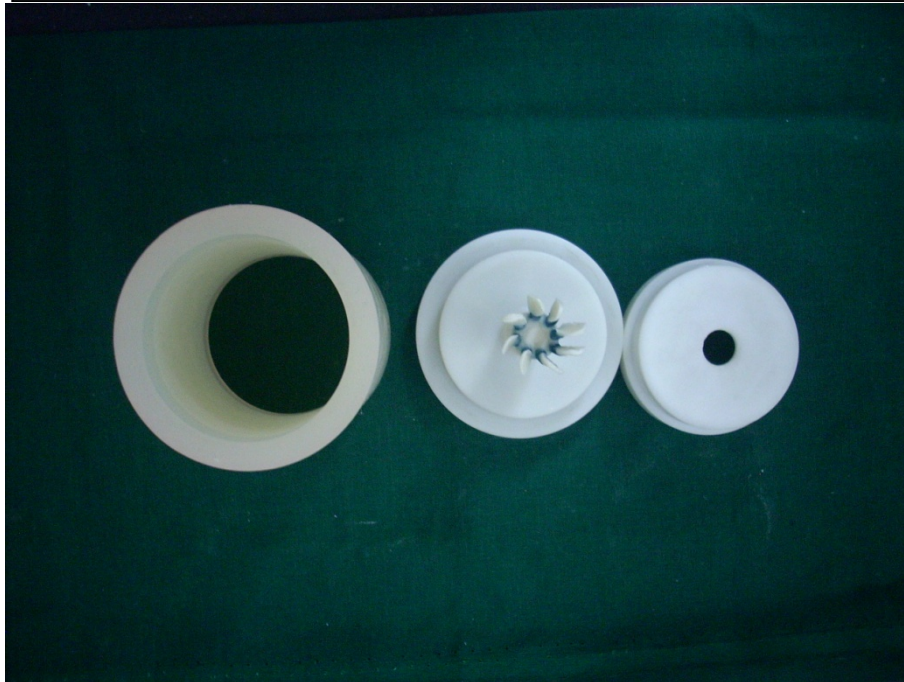
FIG. 9 WAX PATTERN SPRUED
