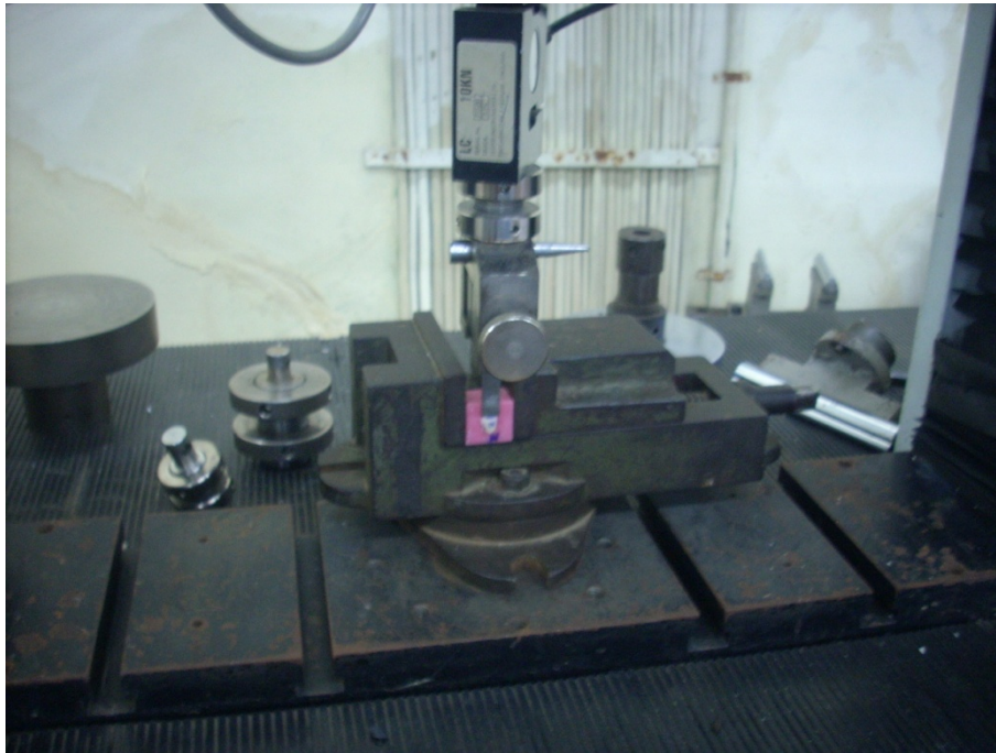
FIG. 28 SHEAR LOADING OF TEETH SAMPLES USING UNIBEVEL CHISEL IN UNIVERSAL TESTING MACHINE
