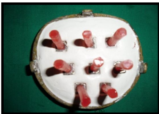
Fig.54: Invested waxed-up alloy samples
