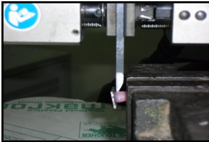
Fig.61: Sample fixed to the sample fixture of Universal Testing machine
