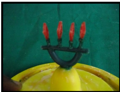
Fig.51: Patterns aligned vertically and sprued to a horizontal bar
