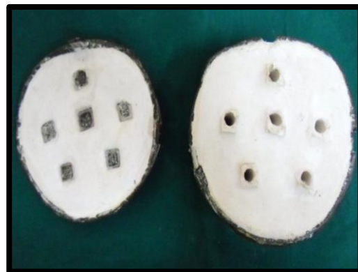
Fig.55: After dewaxing, invested alloy samples in flask base cylindrical mold spaces in the flask body
