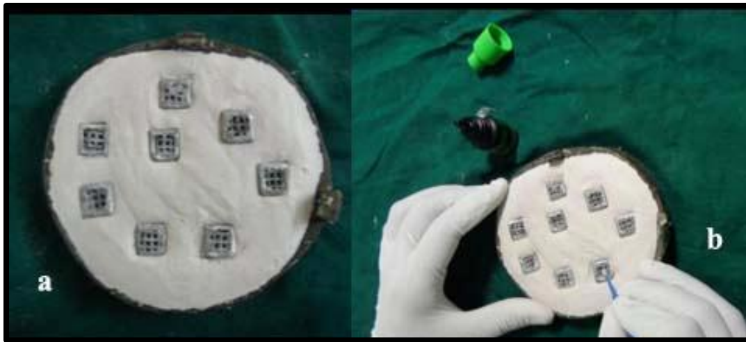
Fig.56a: Air abraded samples, 56b: Alloy Primer application
