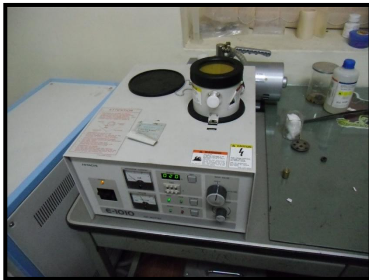
Fig.63: Samples in the gold sputtering machine prior to SEM
