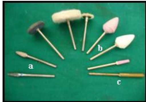
Fig.28a: Metal Trimmers and Mandrel 28b: Acrylic Trimmers, 28c: Sand Paper Mandrel
