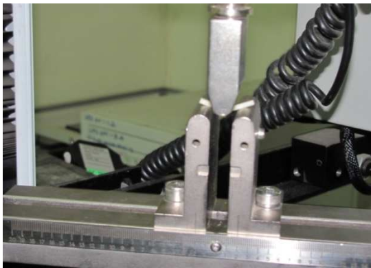
Fig 15–Sample under flexural load
