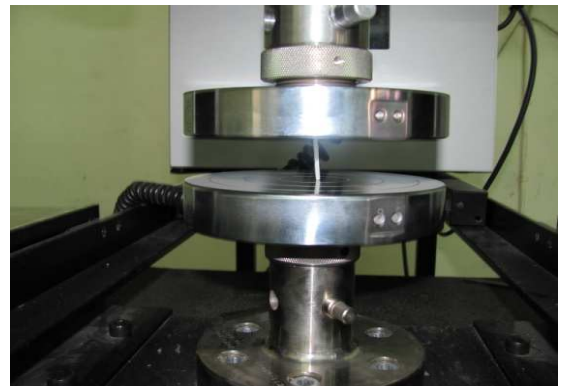
Fig 16–Sample under compressive load
