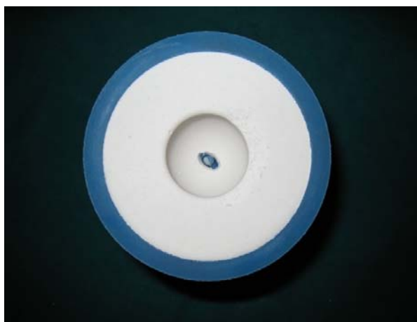
Fig. 14 Sprue former removed
