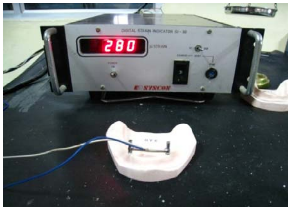
Fig. 74 Bar with strain gauge fixed in open tray sample cast
