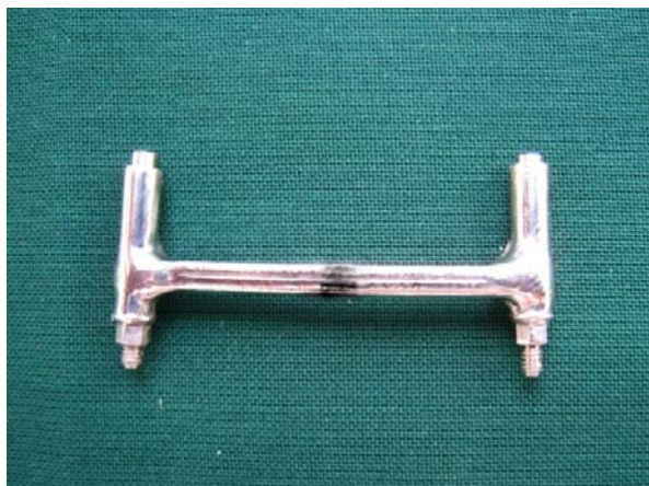
Fig. 19 Laser welded bar
