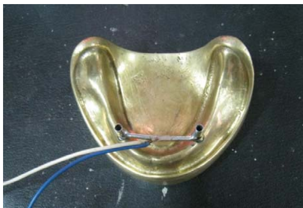
Fig. 71 Bar fixed in master model with strain gage attached
