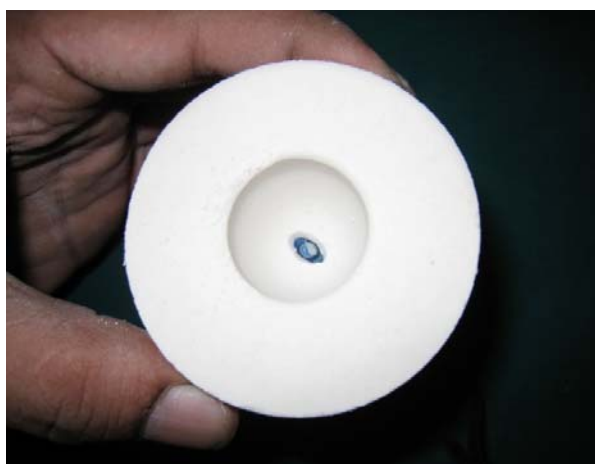
Fig. 15 Casting ring removed for ringless casting
