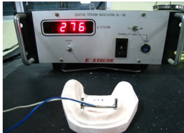
Fig. 75 Bar with strain gauge fixed in closed tray sample cast
