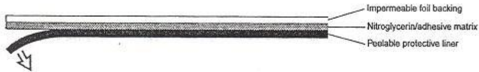
Fig:11-Cross section of Transdermal NTG system:
