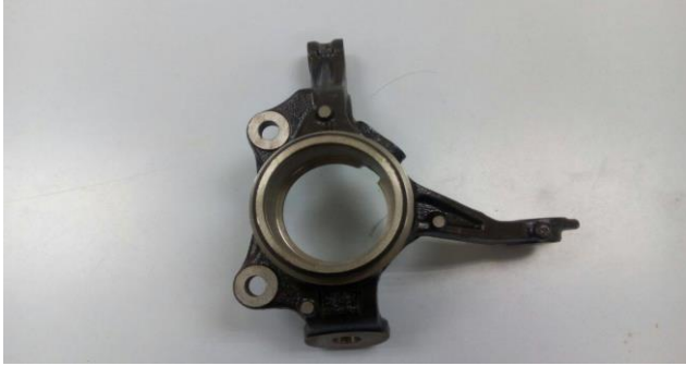
Fig. 1: Actual steering knuckle of 1300 national car.
