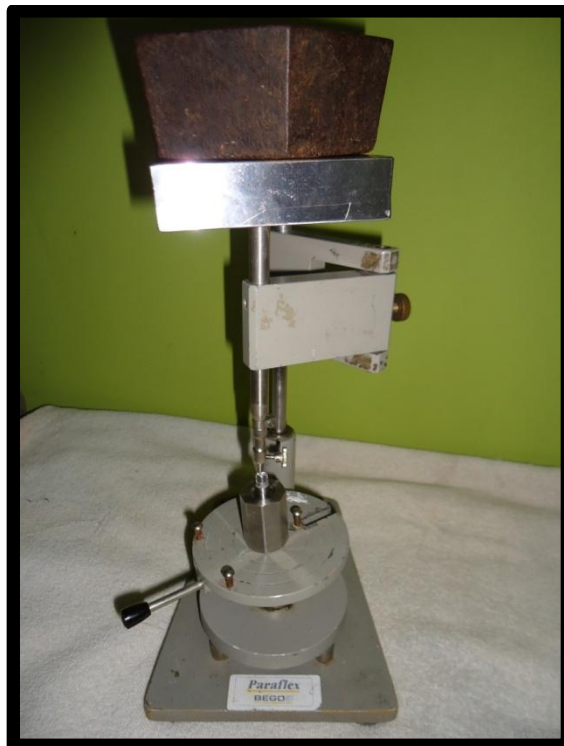
Fig.24: Dental surveyor, (Para flex, Bego Germany) along with custom made platform and 2 kg weight
