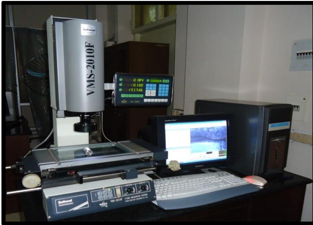
Fig.25: Video Measuring System (VMS2010F)
