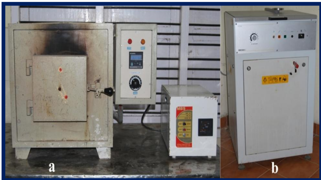
Fig.18a: Burnout furnace b: Induction casting machine
