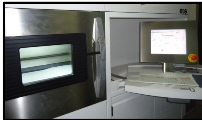
Fig.15b: Direct Metal Laser Sintering Machine
