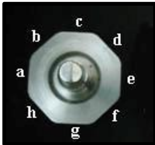
Fig.5a: Schematic representation of 8 predetermined reference areas to be measured for vertical marginal gap
