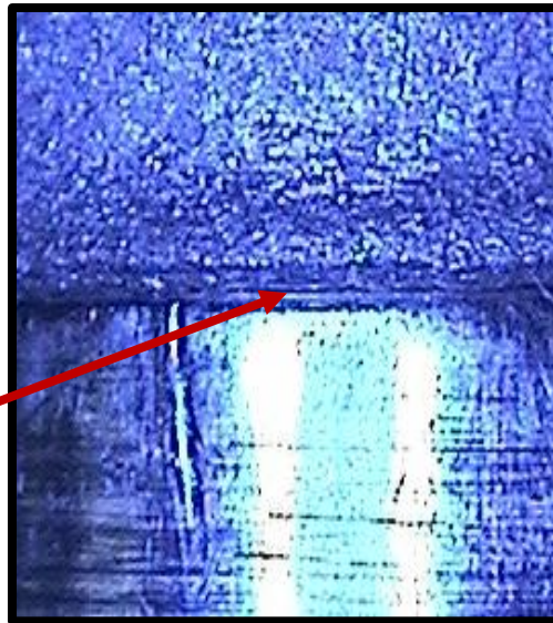
Fig.28: Vertical marginal gap of Co-Cr coping obtained from DMLS technique (G3) as observed under Video Measuring System (VMS 2010 F)
