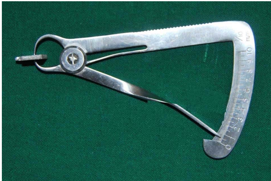
Fig. 16 Thickness of metal substructure
