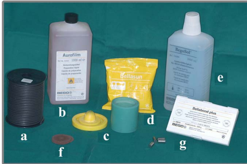
Fig. 7 Materials employed for casting of metal substructure.
