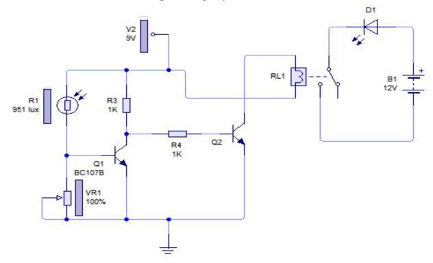
Fig.3. Emergency LED circuit
