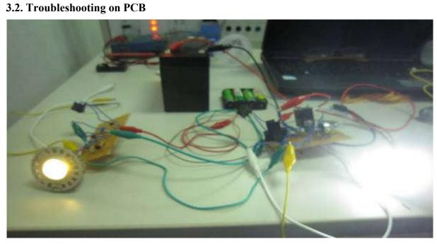
Fig.9. Both 12V LED and 1W LED light up
