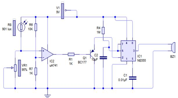
Fig.2. Emergency alarm circuit
