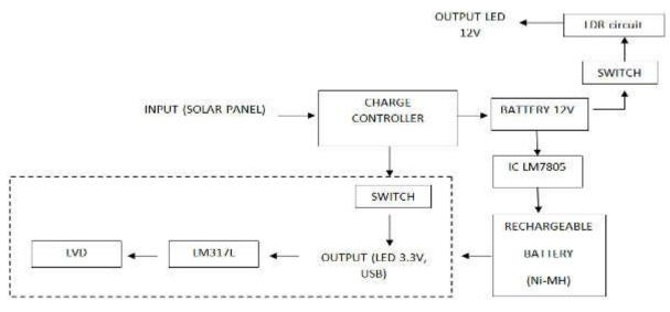
Fig.1. Circuit operation of smart portable solar light
