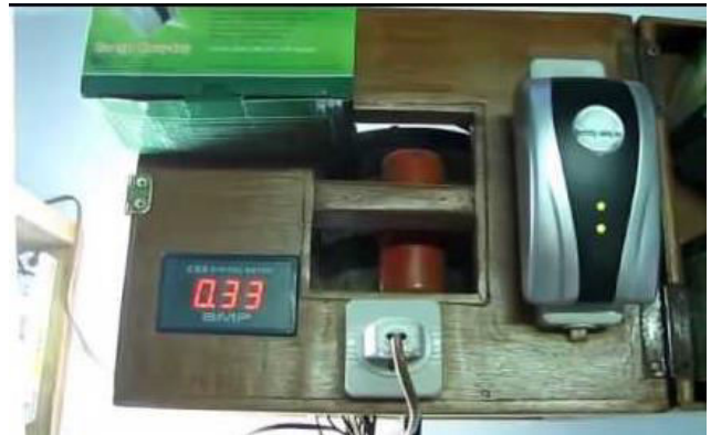
Figure-2. Simulation panel made to show how ESD could reduce the current.
