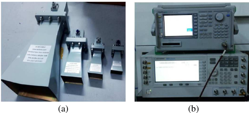
Figure 6. (a) Horn antennas with different effective frequency ranges; (b) spectrum analyzer and signal generator.
