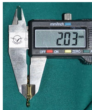
Fig 5, 6: (from left to right) Miniplate thickness measured using digital Vernier Caliper
