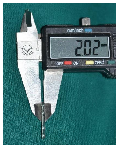
Fig 5, 6: (from left to right) Miniplate thickness measured using digital Vernier Caliper
