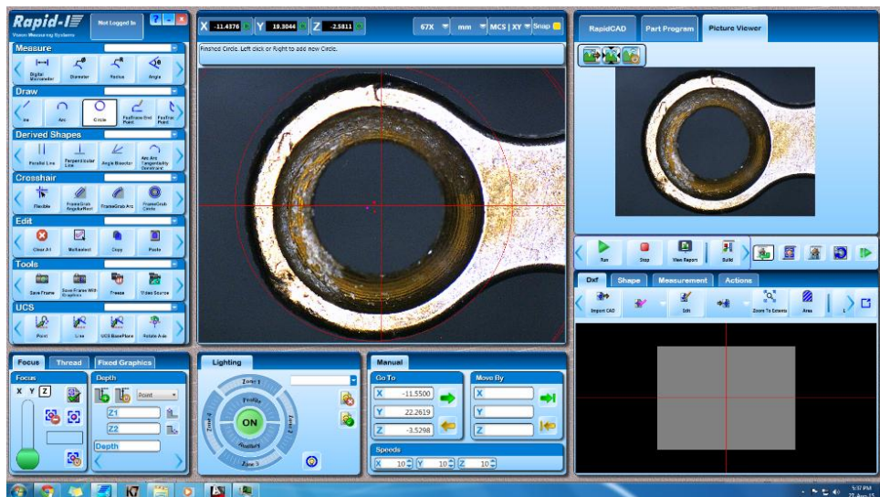
Fig 8: Screen shot of the measurement progress of the miniplate
