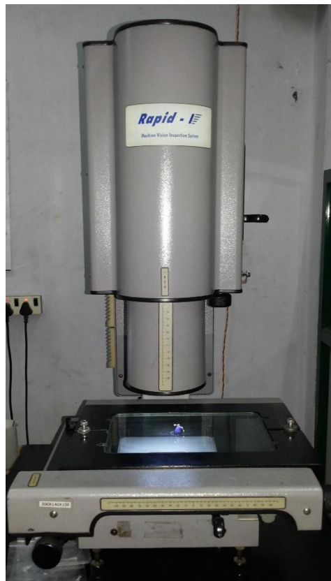
Fig 7: Rapid – I – Vision Measuring System with miniplate
