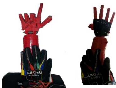
Figure 2. InMoov 3D printed robot with assisted glove.
