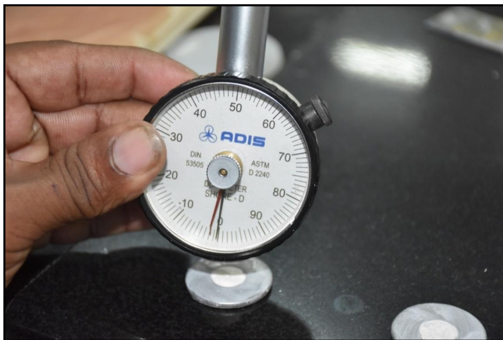
Figure 5: Shore hardness Durometer type A (ADIS Gauges and Tools Manufacturing Company, Mumbai)
