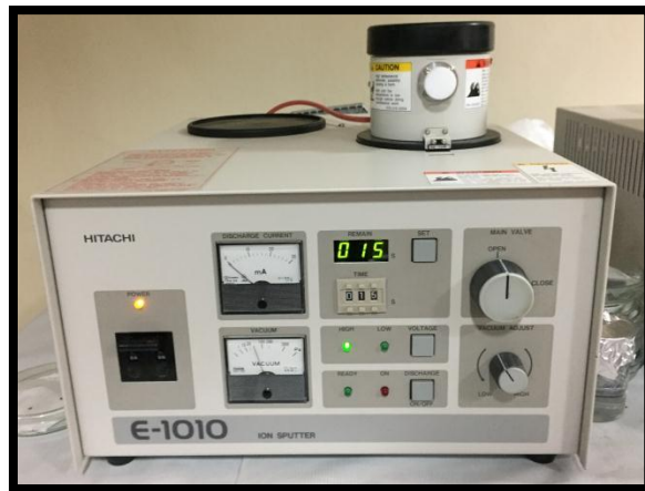
FIGURE 30: GOLD SPUTTERING MACHINE
