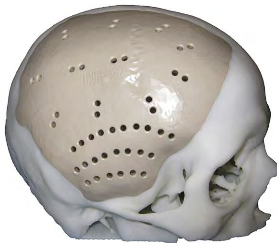
Figure 1.1: Example of a PEEK implant fabricated using milling process
