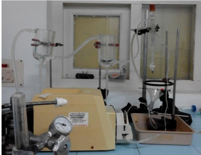
Figure 6: Langendorff perfusion setup
