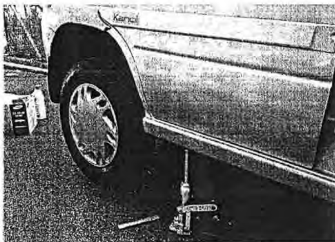
Figure 13. The position of the jack during the lifting of the car.
