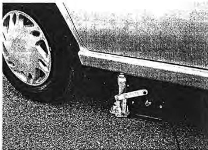
Figure 12. The positioning of the electro-hydraulic jack
