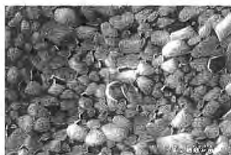
Fig. 7. The HRSEM micrograph of the Zr- containing powders, recombined for 30 minutes at 920°C
