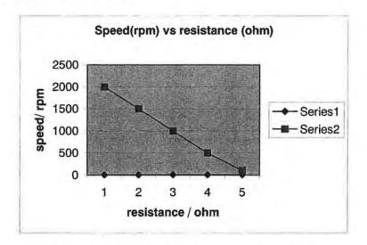
Figure 6 : The results of resistance control experiment
