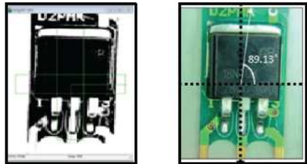
Fig. 5. The rotated image (with flux defect) and image Converted to 8-bit unsigned grayscale
