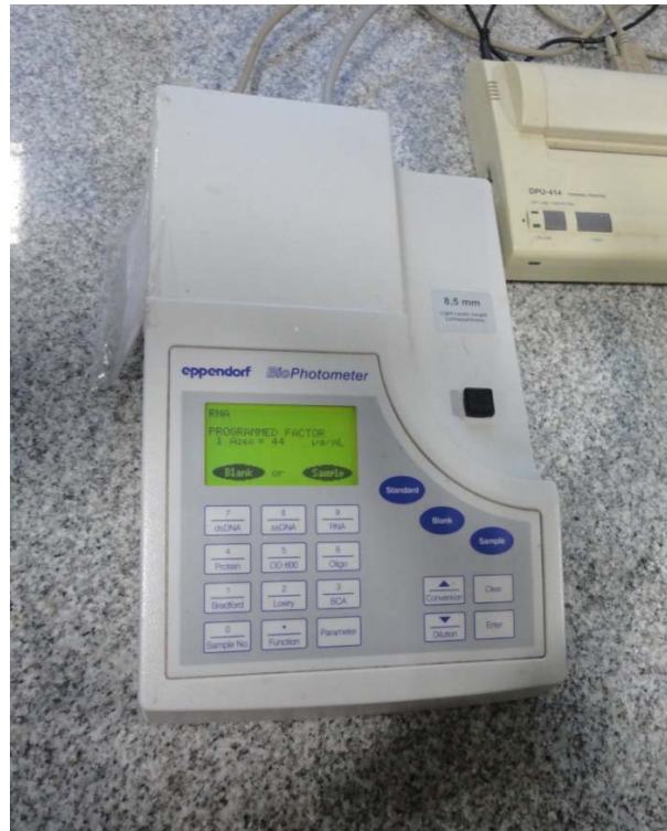
FIGURE 5: EPPENDORF BIOPHOTOMETER TO MEASURE CONCENTRATION OF RNA
