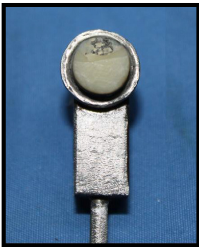
Fig 1.41 Test sample showing cohesive failure
