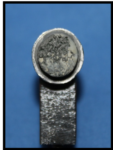
Fig 1.42 Test sample showing adhesive failure
