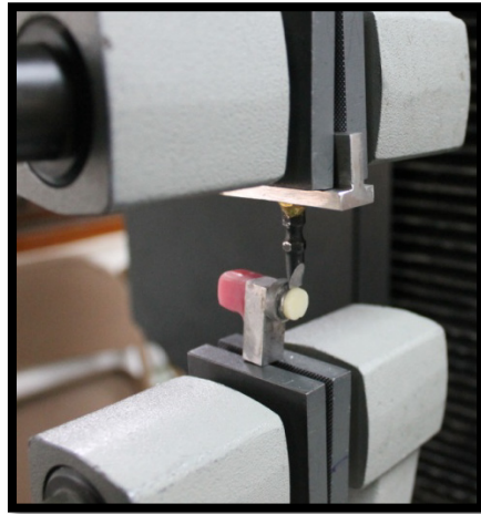
Fig 1.40 Application of shear force in the testing machine
