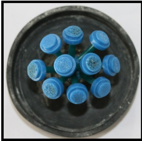
Fig 1.14 Spruing of wax pattern
