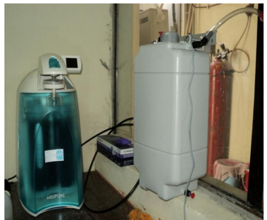
CP21: Machine for deionised water preparation
