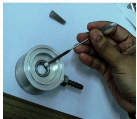
CP9: Test material placed In a die
