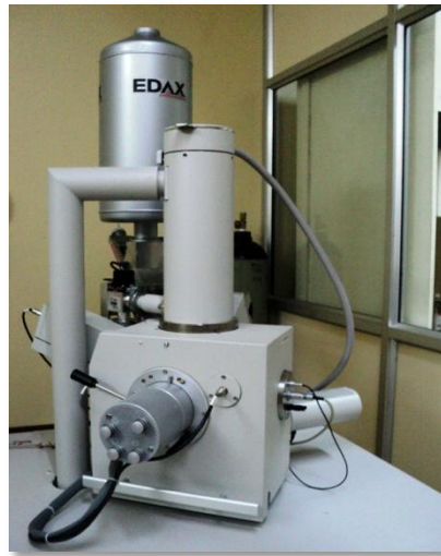
CP 1a: ESEM – Environmental Scanning Electron Microscopy
