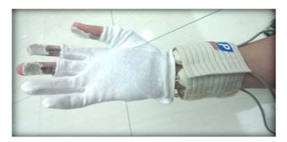
Fig. 2. Complete setup of the sensors
