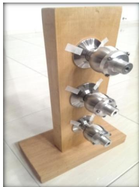
Fig. 6: Loaded Wooden Structure with Knob Adapter and Indicators.
