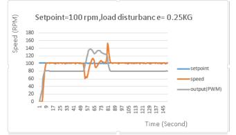
Fig. 27. Closed loop test with load disturbance 0.25 kg
