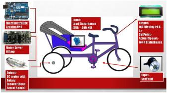
Fig. 5. Conceptual design of trishaw
