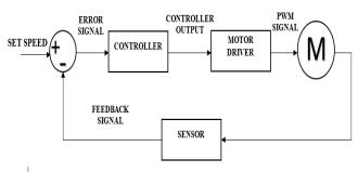
Fig. 3. Closed loop system block diagram.
