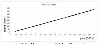
Fig. 11. PWM Input vs Speed of DC Motor (Open Loop)
