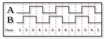
Fig. 9. Two output from rotary encoder represent two square wave in rotary encoder
