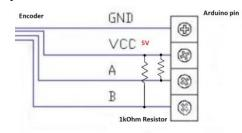
Fig. 8. Rotary encoder connection to Arduino
