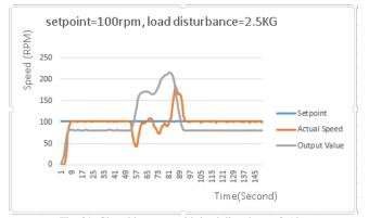
Fig. 29. Closed loop test with load disturbance 2.5 kg
