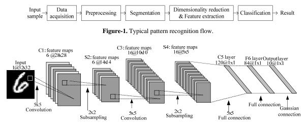
Figure-2. Example of CNN architecture used for handwriting recognition application [1].
