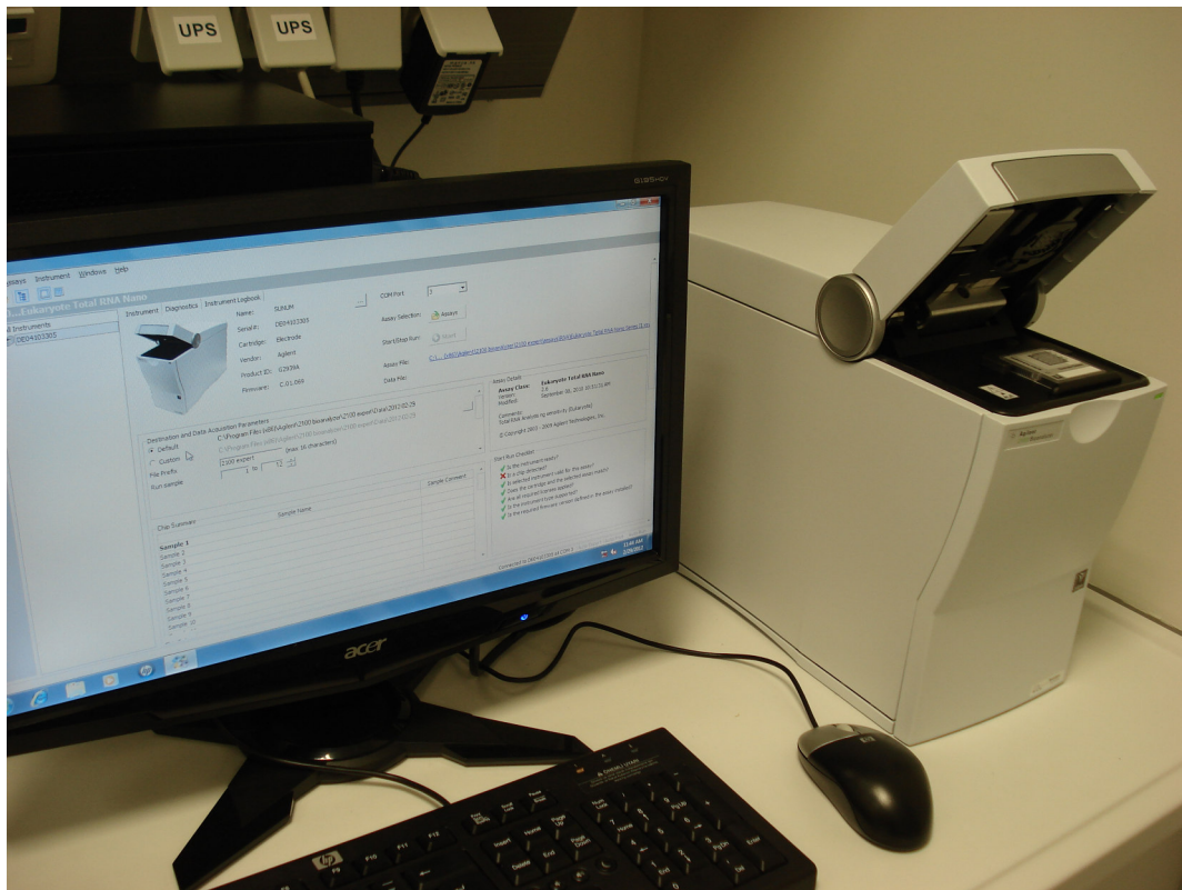
Figure 6.4 Agilent Bio analyzer with complete set up.
