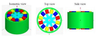
Fig. 7. Structure of S:R = 12:8 poles ratio actuator
