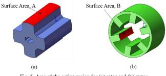
Fig. 5. Area of the active region for (a) rotor and (b) stator
