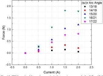
Fig. 13. FEM result of force characteristic for varying arc angle for S:R = 12:8 poles ratio when air gap thickness is 0.2 mm
