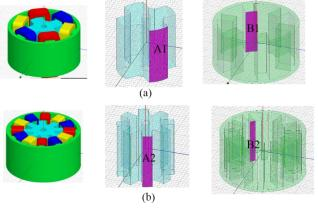
Fig. 11. Area of active region for S:R poles ratio (a) 6:4 and (b) 12:8
