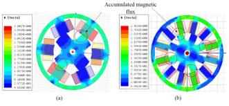
Fig. 10. Distribution of magnetic flux for S:R poles ratio (a) 6:4 and (b) 12:8
