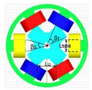
Fig. 2. Geometrical dimension of the arc angle for S:R = 6:4 poles ratio
