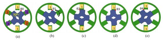
Fig. 3. Rotor position to derive the inductance profile
