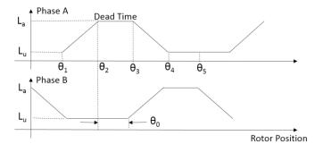
Fig. 4. Typical overlapping inductance profile
