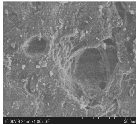
Fig. 7.17 : Membrane Morphology of Formulation F04C2 by Scanning Electron Microscope
