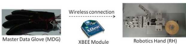
Figure 4 Schematic diagram of developed prototype
