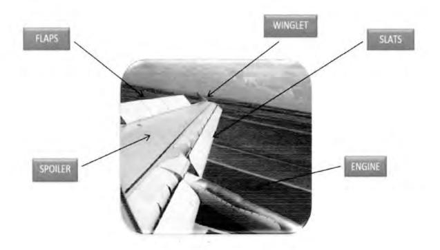
Figure 1.1 Aircraft slat and flap (Sahin, 2012)
