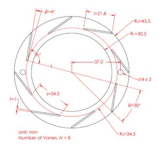
Figure 1: Dimension of diffuser with 8 vanes.
