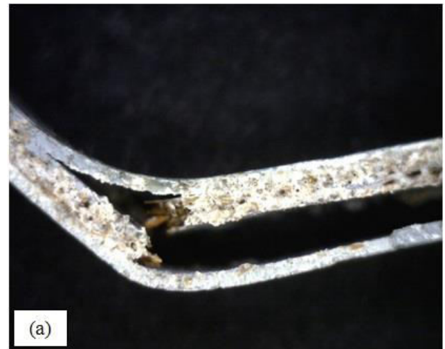
Figure-9. 30wt% OPEFB fibre FML (a) Flatwise impact; (b) Edgewise Impact.
