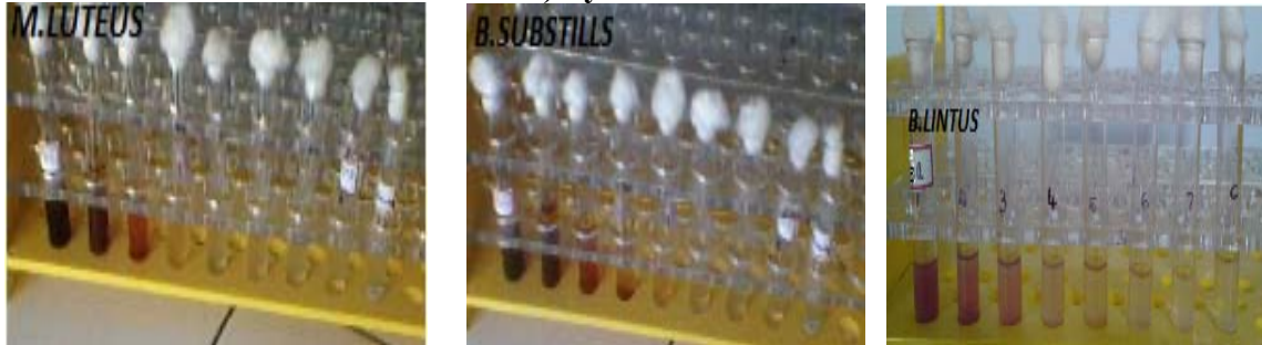
Figure 15. Minimum inhibitory concentration of synthesized compounds (gram positive strains) by serial dilution method
