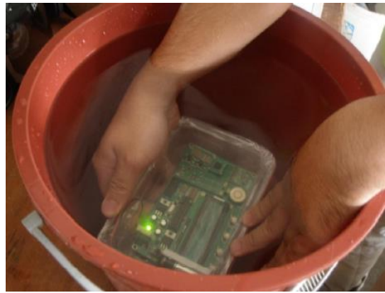
Figure 4(c) PR22 Board was Immersed in the tap water
