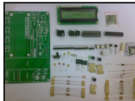
Figure 3(a) PIC board before combining all the components
