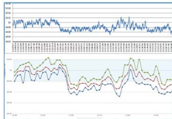
Figure-4. Real time data feed (T. Gobmaier, 2011) and the data from Arduino (minimum, average and maximum).
