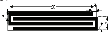
Figure 4: Schematic and dimensions of the proposed Halfring AMC structure where m = 29 \text{ mm} , n = 4 \text{ mm}
