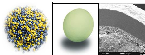
Figure 2: 1. Pellets, 2. Perfect pellet, 3. Coated pellet
