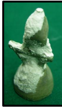
Fig.36b: Partially cleaned casting
