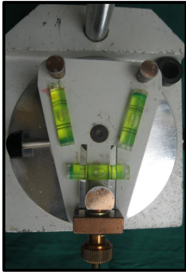
Fig.26: Surveying platform made parallel to the floor using spirit level indicators
