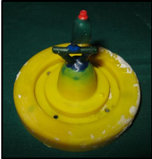
Fig.35a: Pattern attached to crucible former
