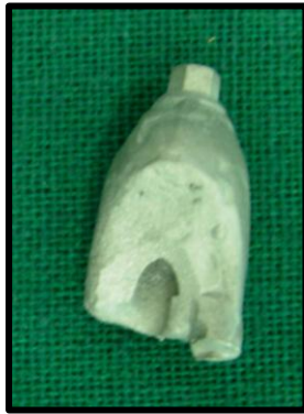
Fig.36d: Casting after sprue sectioning
