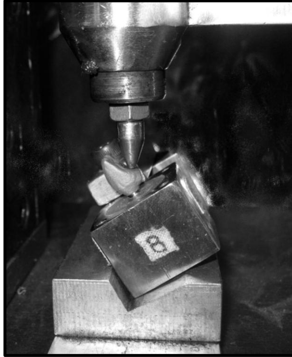
Fig.42a: Stylus placed on flattened cingulum of test sample
