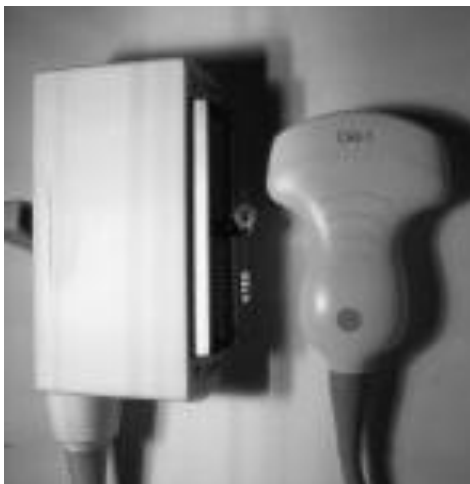
Siemens CH4 – 1 convex probe - Two dimensional color Doppler sonographic probe
