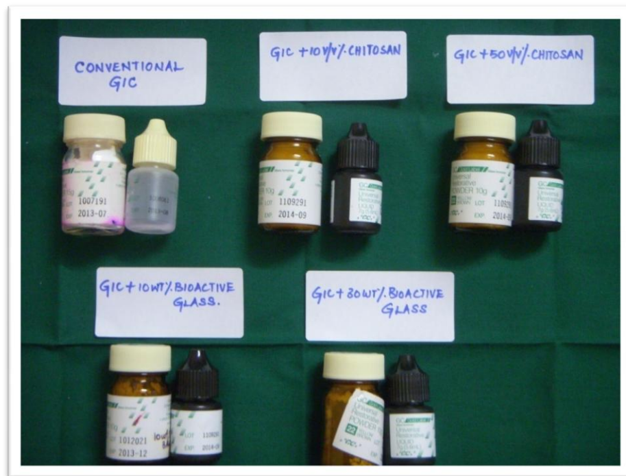
Fig.2 GIC, GIC+Chitosan (10v/v% & 50 v/v%), GIC+Bioactive glass(10 wt% & 30wt%)
