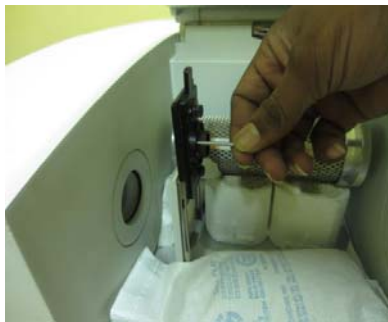
Placing the carrier into the FTIR spectrometer
