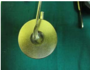
KBr powder pouring into the bore of the die section
