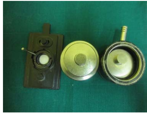
Transferred KBr pellet to the FTIR carrier
