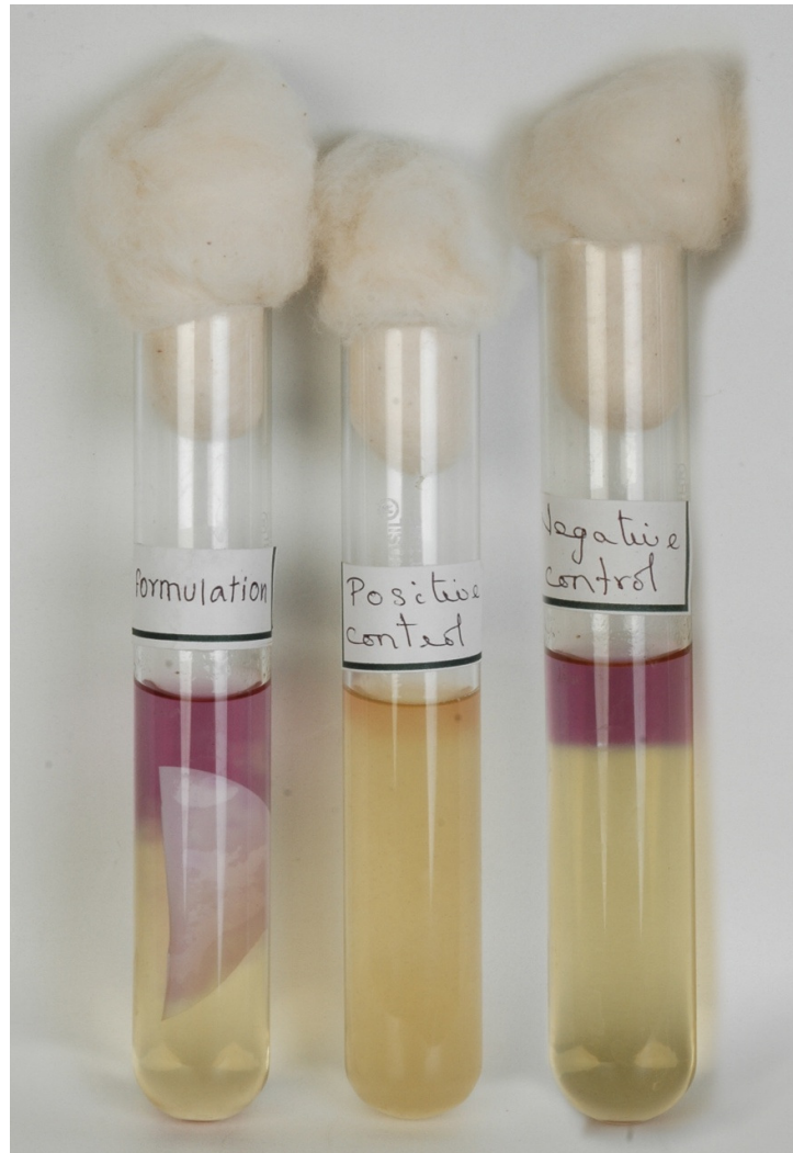
Fig: 22: Observations of sterility test done in Fluid Thioglycolate medium (FTM)
