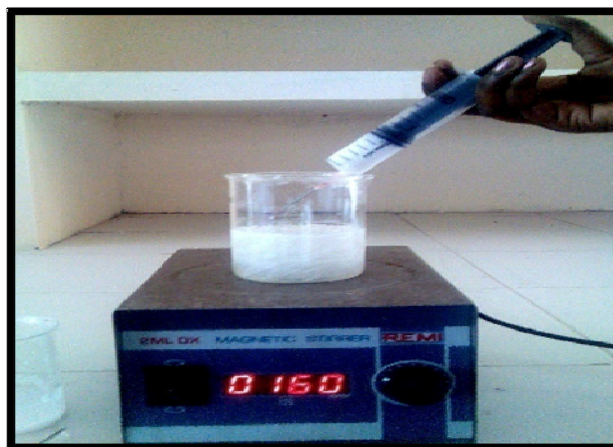
Figure.7.2: Preparation of microspheres using 22# syringe needle in magnetic stirrer
