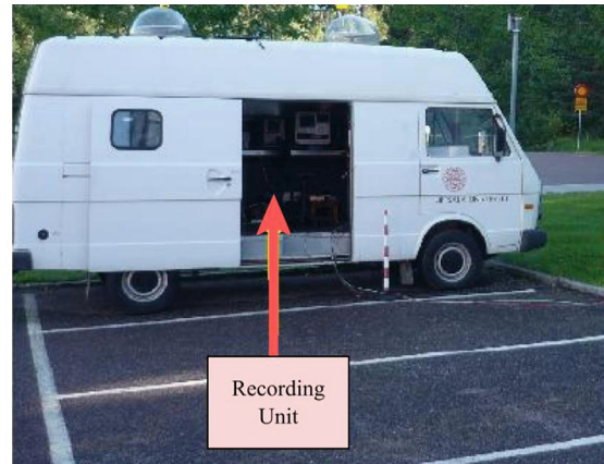
Fig. 1. The measurement instruments are placed within fully grounded and protective metal van.
