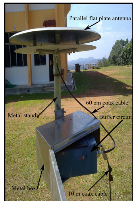
Fig. 2. An electric field change recording system located about 9 m from the observatory station building. The buffer circuit was shielded in a metal box during measurements and the captured electrical signal was directed through the 10 m coaxial cable to a DSO located inside the observatory station building.
