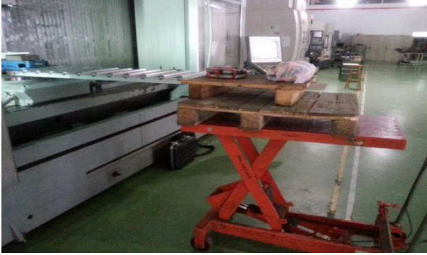
Fig. 4 Roller conveyor attached to the CNC machining centre
